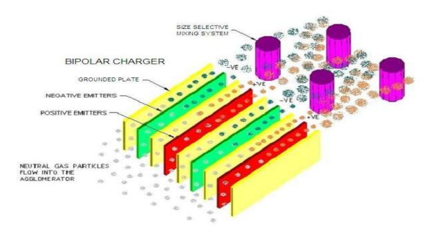
Figure 4. - The Bipolar Electrostatic Agglomeration Process (BEAP)
