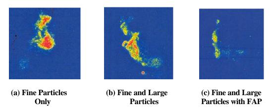
Figure 3. - Color Coded LIF Analysis of Fine Particle Mass Density
