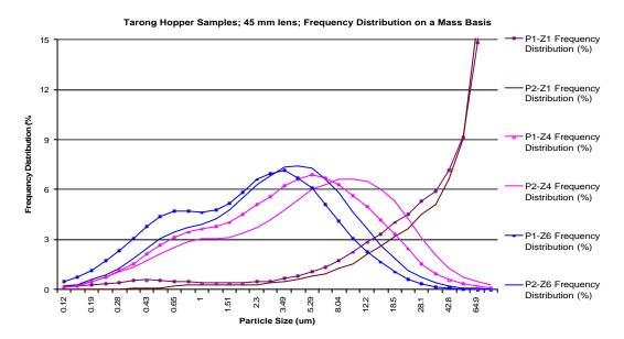
Figure 6 – Hopper Particle Size Distribution
