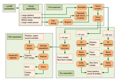
Fig. 4. General flow sheet of the intended material recuperation process within the CtC project.
