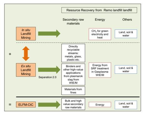
Fig. 2. Resource recovery from *in situ* and *ex situ* landfill mining – the double arrow indicates that for the Closing the Circle (CtC) project an *in situ* LFM phase (on landfill cells that are not excavated yet) can be combined with *ex situ* LFM (on landfill cells that are excavated).
