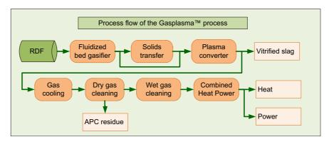
Fig. 5. Overview of the Gasplasma<sup>TM</sup> WtE/M process (RDF = Refuse Derived Fuel = SRF = Solid Recovered Fuel, Vitrified slag = plasmarok, APC = air pollution control).
